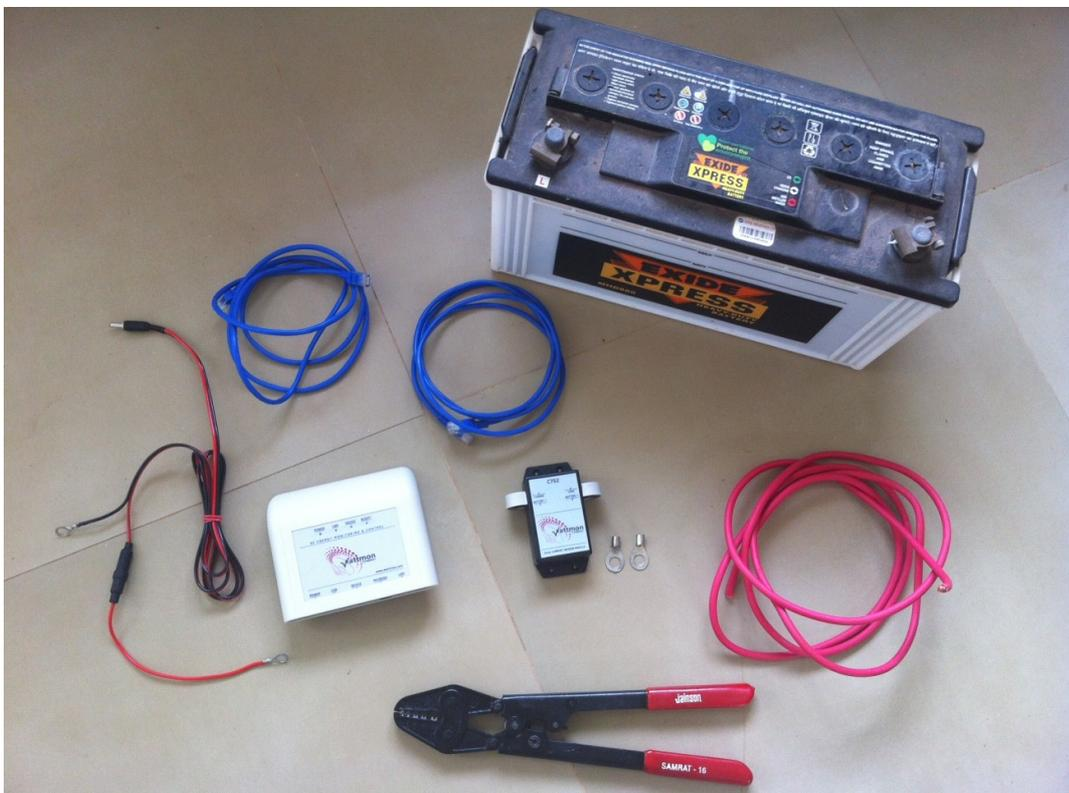
*Figure 1.1 Wattmon components prior to hooking up with the battery*
