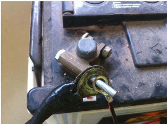
Loosen the negative battery terminal (black one, marked with a - ) and remove the nut. Fix on the black wire of the wattmon power cable to this and re-tighten.
