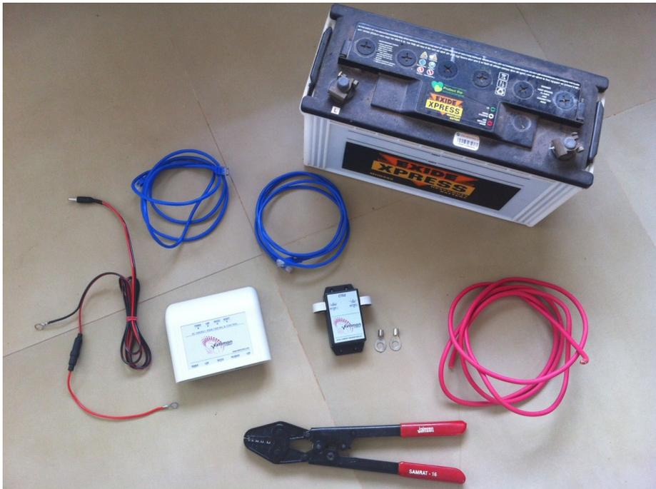
Figure 1.1 WattmonSolar components prior to hooking up with the battery
