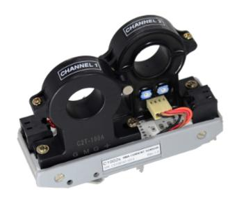
The current transformers are a bidirectional, hall effect, open loop device based on the measuring principle of the hall effect, with a galvanic isolation between primary and secondary circuit. It provides accurate electronic measurement of DC currents in the range of  $0-\pm150$ . The loop hole size is 21 mm.
