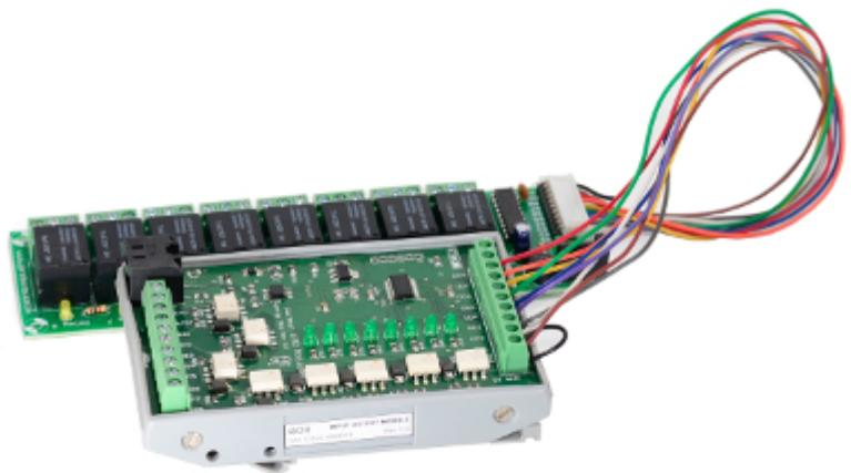
It can be configured and controlled by any Modbus RTU master device over RS-485.
