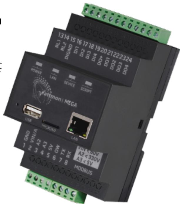
The MEGA uses the same OS as any of the Wattmons including the PRO, and is compatible with the same set of Modules and Accessories. The firmware has the same set of functions as all of the Wattmons and the PRO, but is expanded to take advantage of the hardware improvements. These changes add flexibility and speed, making it over twice as fast as the PRO and easier to customize for any application.
