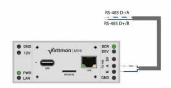
For most applications only the RS-485 A and B lines need to be connected to the device to be monitored and controlled. For example, all the Wattmons have drivers for these inverters, and many more:
