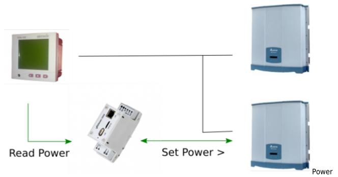
control signifies dynamically changing an Inverter's output power based on an algorithm. Wattmon supports dynamic power control using an add-on software package and can be used in conjunction with a power meter for various purposes:
