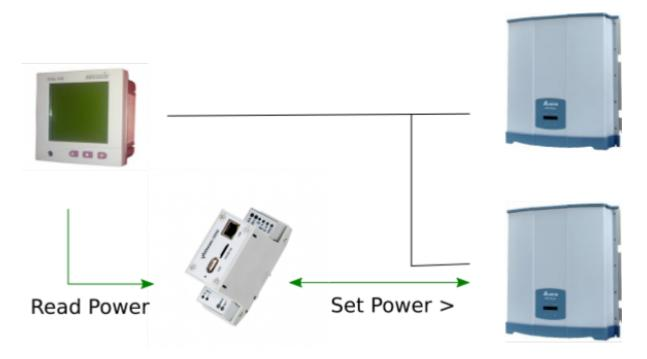
Power control signifies dynamically changing an Inverter's output power based on an algorithm. Wattmon supports dynamic power control using an add-on software package and can be used in conjunction with a power meter for various purposes:
