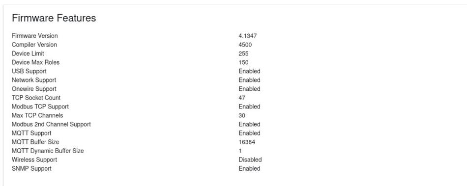
The second section shows the firmware and configuration values currently loaded. This indicates the maximum values. For example the above shows that Wattmon supports a maximum of 30 Modbus TCP channel, and supports device drivers with 150 roles.
