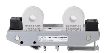
The current transformers are a bidirectional, hall effect device based on the measuring principle of the hall effect, with a galvanic isolation between primary and secondary circuit. It provides accurate electronic measurement of DC currents in the range of 0—±25. The loop hole size is 8 mm.
